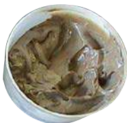
Used grease: colour turned greyish
