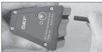
Fig 2 Fitting or removal of V-guides
