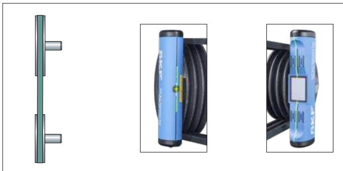
Figure 9 Pulleys perfectly aligned
