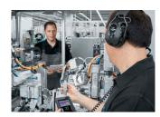
Systematically identifying leaks in compressed air systems and professionally eliminating them considerably reduces compressed air costs, because leaky compressed air components waste lots of energy and money. Our specialists check the entire compressed air system – from the compressor to the pneumatic application.
