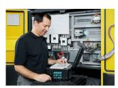
Monitoring the compressed air generation over several days, including downtimes and the weekend, produces a clear consumption profile. It documents the power and compressed air requirements including fluctuations in consumption from basic load to peak load at different times of operation. The savings potential is then outlined in a report.
