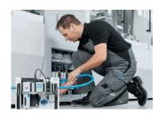
When measuring the precise compressed air consumption at the individual machines at rest and during operation, our team analyses various parameters such as consumption per machine cycle, average consumption per minute, average pressure, maximum/minimum pressure and maximum/minimum air volume flow. These measurement results are documented in a report.
