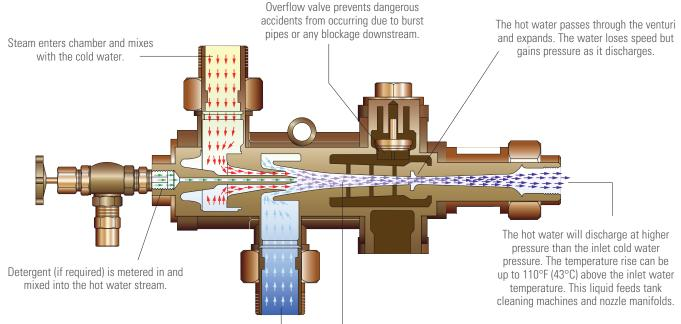
The cold water instantly condenses the hot steam and creates a vacuum. The cold water absorbs the heat and velocity from the steam and a high-speed stream of hot water is produced.
